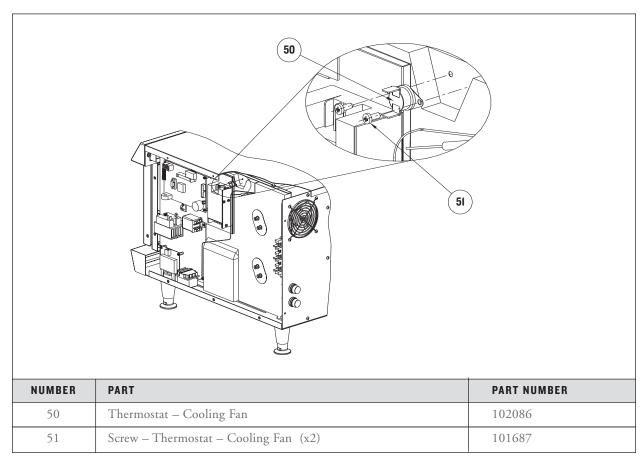
FIGURE 48: Removing Cooling Fan Thermostat
